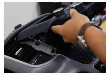
**Step 11:** Flip bezel over and start putting the T15 screws back into place.
