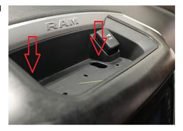
**Step 2:** Pull bezel/radio forward, carefully disconnect all the connections for the radio and bezel. There could be up to nine connections.
