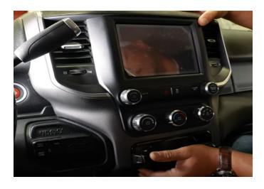
**Step 17:** Reinstall the two T20 Torx screws you placed to the side. Then plug new tray cover in place.
