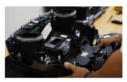
**Step 6:** Remove the screws around the factory radio and plastic bracket.
