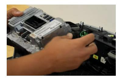
**Step 8:** Remove the T15s from the inner bezel.
