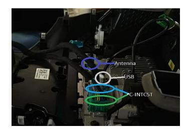
**Step 15:** Make the rest of the connections to the radio & bezel.
