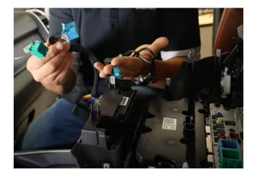
**Step 14:** Connect the included three harnesses to the rear of the radio.
