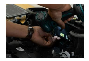
**Step 9:** Flip the bezel over and remove the inner bezel.
