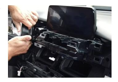
**Step 39:** Reinstall the upper dash. Remember to connect your hazard switch then push the upper dash into place. You'll hear the clip from the retainer clips engaging.
