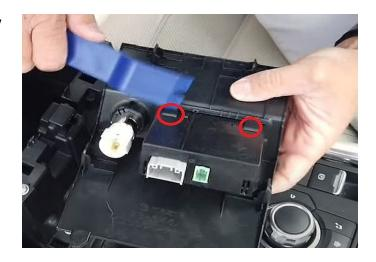
**Step 45:** Slide the new USB hub into the panel.
