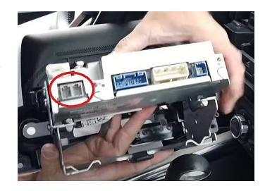
**Step 35:** Plug in all six connections at the rear of the radio then slide it back into place in the dash.
