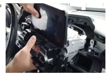
**Step 29:** Pull the radio out enough to disconnect the rear connections. There is a small locking tap at the top of each connection. Press down to release lock.
