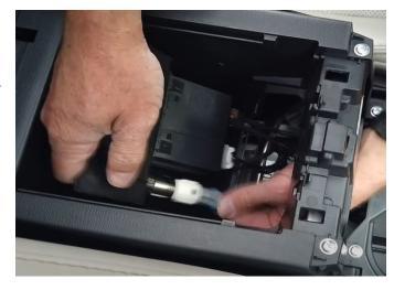
**Step 50:** Slide the USB panel into place. There are two tabs at the bottom that need to be hooked then the panel leans forward.
