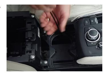
**Step 48:** Bundle up any excess from the USB cables, zip tie the cables and put the excess under the cup holder cavity.
