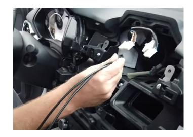
**Step 32:** Pull the slack down to the driver's foot well.
