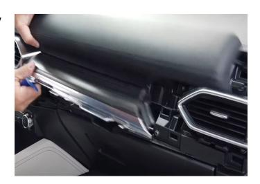
**Step 24:** Disconnect the hazard button then set the upper trim panel off to the side.
