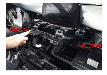
**Step 26:** Next remove the two 10mm bolts holding the radio in place.
