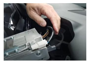
**Step 30:** Time to run the two included USB cables into the dash and down to the driver's foot well. The brown and black connector goes to the new USB hub. The end with the green tipped connectors goes to the rear of the radio.
