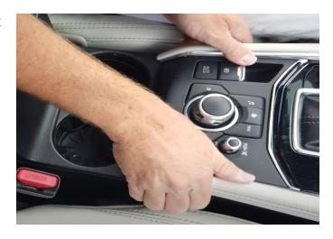
**Step 42:** Next remove the cup holder trim, it is only held in with retainer clips. Place it off to the side.
