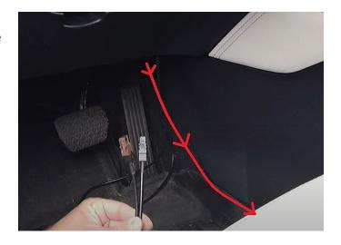
**Step 47:** Route the cables under and through to under the cup holder. You can pull all the slack through.
