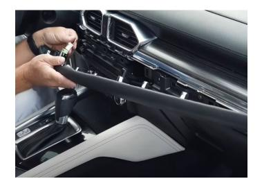
**Step 41:** Next let's install the new USB hub. First pull up on the shifter trim panel. It is only held in with retainer clips. You do not need to remove it fully, pull up enough to give you more room to work.
