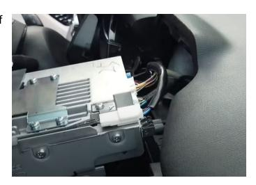
**Step 36:** Reinstall the two 10mm bolts you removed earlier.
