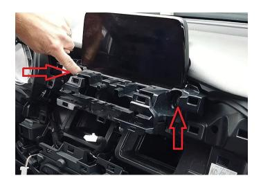
**Step 27:** Before you can slide the radio out. Pull the cluster bezel's corner up a bit to allow the radio to release from the dash freely.
