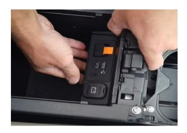
**Step 51:** Reinstall the cup holder, push it down to hear the retainer clips snap into place.
