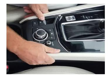
**Step 53:** Start the vehicle in accessory mode for one minute. Then turn the vehicle off. Insert the Map SD card into the new USB hub's SD Map card slot.
