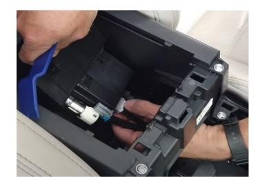
**Step 44:** There are four tabs holding the factory USB hub in place, two on top and two on bottom. These need to be pressed in to release the hub.
