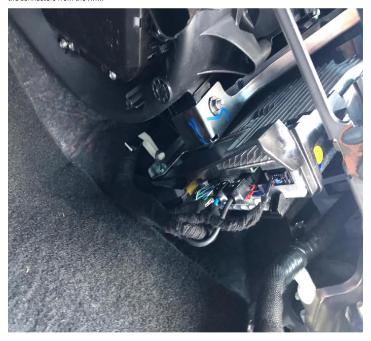
Step 4: There are 2 screws that you need a size 7mm socket to get them out. This way you can move the bracket holding it in. Pull the carpet back and pull out the original HMI. There are 2 levers holding it from falling that you need to push back for it to come out.
