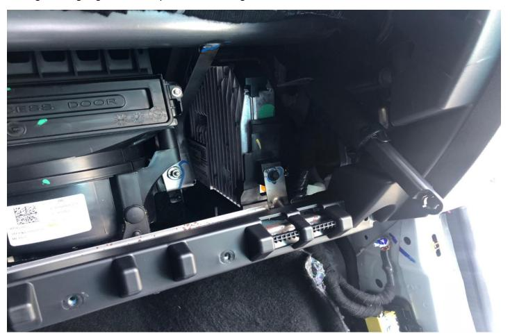
Step 3: You will see your original HMI right there on the right. All the connectors have tabs you need to release with a tiny flat head screwdriver, so you can get the connectors out. Some are red and some white. Release all the connectors from the HMI.
