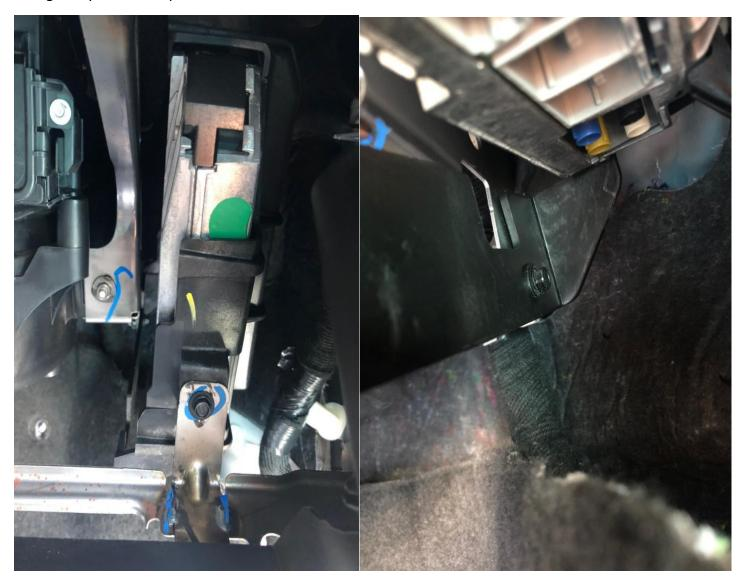
Step 5: Install the new HMI we provided you with from Infotainment.com that has Navigation. Move the bracket back into place. Reconnect all the connectors. Put the 2 screws back into the holes. Re Install the glove box first pushing it into the bars at the bottom then connecting the rod that was holding it up then pushing it closed.
