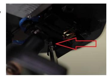
**Step 5:** Take the new digital rear view mirror and plug in the factory connector.
