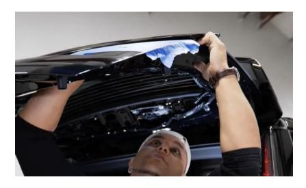
**Step 35:** Once the clips are released, you'll need to disconnect the factory backup camera and push button connections. Push red locking tab out then disconnect plugs.
