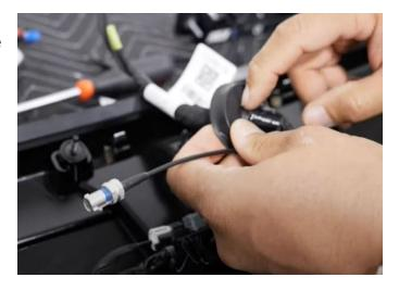
**Step 44:** Plug in your last connector then push the red locking tab down.
