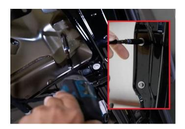
**Step 48:** Time to reinstall the large panel with the close lift gate button. Reconnect the close lift gate button. Make sure to push the locking tab back down.
