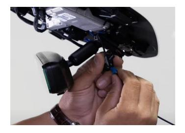
**Step 8:** Push the plastic clip on the female fakra from the mirror into the hold to the right of the silver module. This will secure the cable into place.
