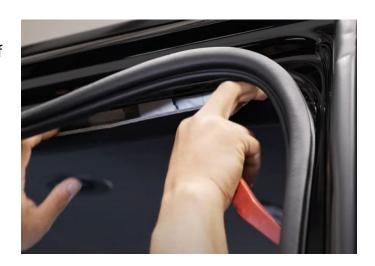
**Step 18:** Now in the rear keep routing the cable back and under the headliner.
