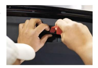
Step 27: You can now pull down the large trim panel, it is only held in with retainer clips and the close button will still be attached when all clips are released. You want to start at the window and work down. You want to pop the lower part of the panel down then out at the same time.
