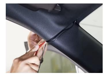
**Step 14:** Pull down your door's weather stripping to gain access to route the fakra cable toward the rear of the vehicle.
