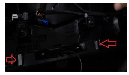
**Step 39:** Remove the two T15 screws then move the factory backup camera over to the new housing.
