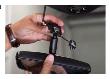
**Step 6:** Slide the new digital rear view mirror into place and secure with the T20 screw.
