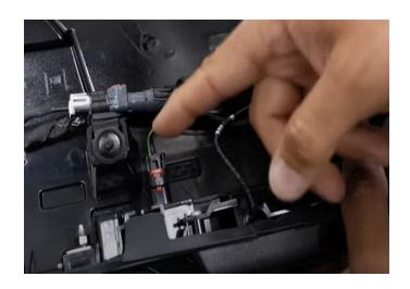
**Step 45:** To reinstall the valance, feed the camera cable through the factory hold. Reattach the grommet then line panel up and push till you hear retainer clips snap into place.
