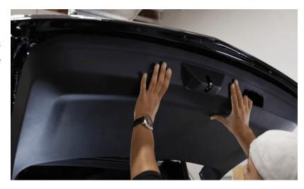
**Step 50:** Reinstall the corner trim panels. You'll hear the retainer clips snap into place.
