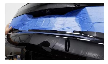
**Step 33:** Next we need to remove two 8mm screws from each side, four total. The screws are sliver. Then remove the eight 8mm nuts. These are black. Some are quite easy to see, some are a bit more hidden inside the circle cutouts.
