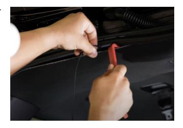
**Step 21:** Pull the left grommet down then use a long zip tie to feed into the grommet till it reaches above the headliner.
