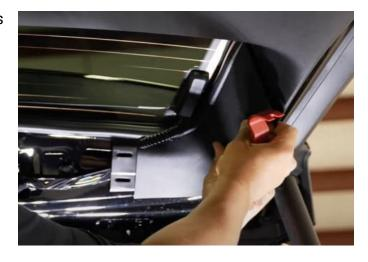
**Step 26:** Moving to the handle, remove the plastic trim hiding the 7mm screw. Remove the screw and place to the side.
