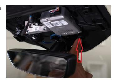
**Step 9:** Run the fakra cable up to the top of mirror assembly, use zip ties to secure wiring.
