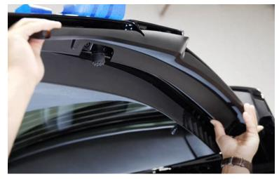
**Step 53:** Reinstall the 7mm screw then the handle screw cover.
