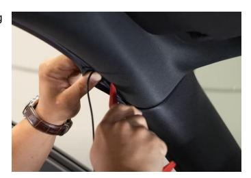
**Step 15:** Continue down to the end of the driver's door. Once wire is in place, reinstall the weather stripping.
