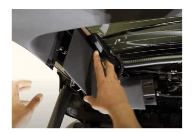
**Step 51:** Reinstall the center trim panel. You'll hear the retainer clips snap into place.
