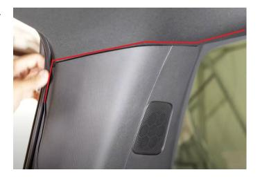
**Step 20:** Open the rear lift gate, pull the weather stripping down and route the cable above the head liner.
