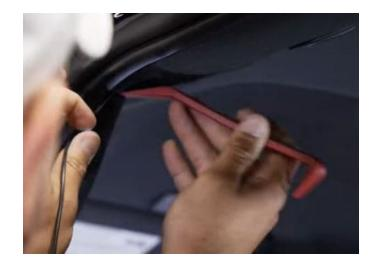
**Step 17:** Remove rear passenger door weather stripping then route the cable toward the rear of the vehicle.
