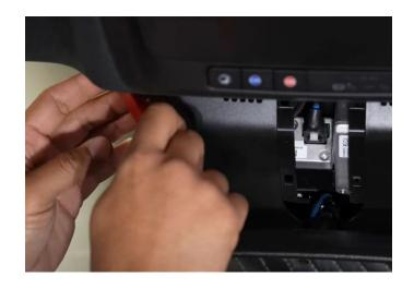
**Step 3:** Angle the factory mirror down and disconnect the one black connector going to the mirror.
