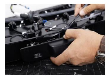
**Step 41:** Reinstall the two 8mm nuts.
