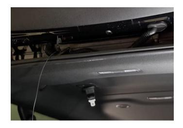
**Step 24:** Start by popping off the top panel, use your pry tool in the corner to start popping out the retainer clips. Place the panel off to the side.
