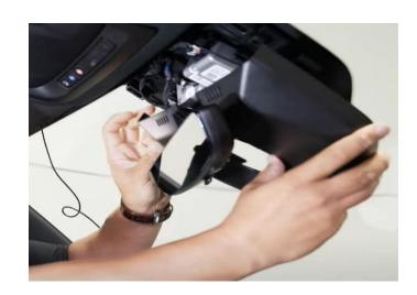
**Step 12:** Reinstall the rear view mirror smaller trim panel back into place.
