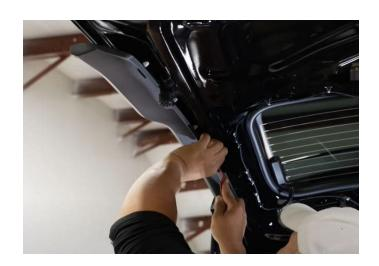
**Step 30:** With the panels removed, you can feed the fakra cable up into the lift gate. Reattach the factory rubber grommet.
