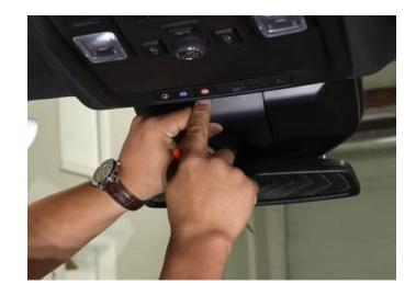
**Step 2:** Next, using your pry tool, pull down in the top left corner of the trim panel. Do not put any force on the glass, it doesn't take much to crack the windshield. The panel is only held in with retainer clips.
