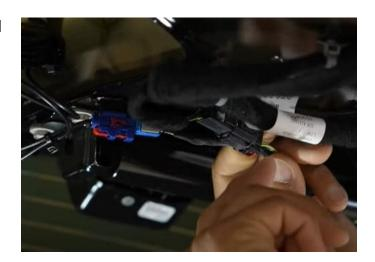
**Step 36:** With one hand support the valance and the other hand pull the wiring and grommet out of the lift gate.
