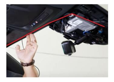
**Step 11:** Reinstall the rear view mirror trim panel. You'll head the retainer clips snap into place. Make sure not to pinch any cables.
