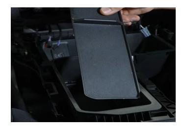
**Step 9:** There are three 10mm bolts holding the cubby in place. Remove the cubby and place to the side.
