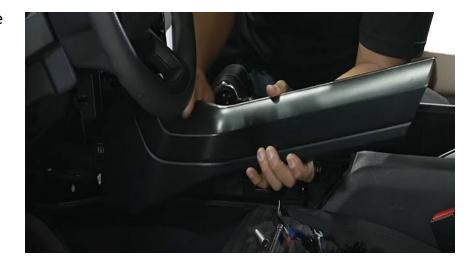
**Step 32:** Install the dash trim under the radio controls.
