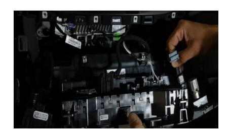
**Step 30:** Install the four 7mm screws back into place.
