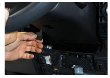
**Step 17:** Remove the three 7mm screws from the bottom of the steering wheel column.
