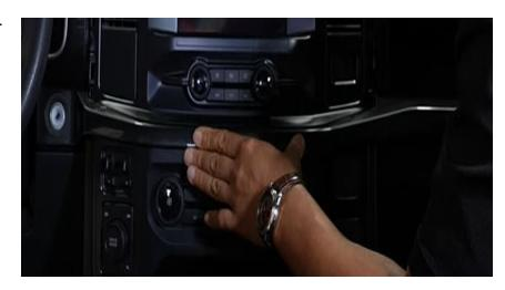
**Step 33:** Install the trim panel above the radio screen.
