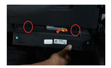
**Step 15:** You can now remove the knee bolster as it is only held in with retainer clips.
