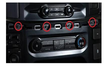
**Step 5:** Once the four screws were removed you can pull the HVAC controls.
