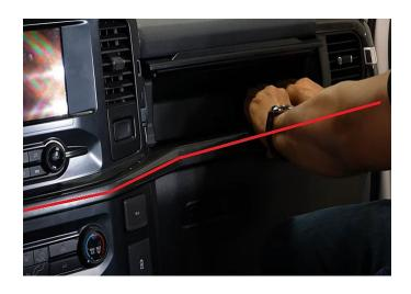
**Step 3:** Open the center console armrest then remove the trim panels on both sides of the center console. Start pulling to the side the part of the panel closest to the armrest. Panel is only held in with retainer clips.
