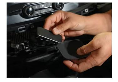
**Step 14:** Next you need to remove the knee bolster. Start by pulling the bottom panel down to expose the two 7mm screws.
