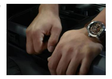
**Step 8:** Remove the floor of the cubby and the rubber mat.
