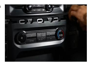
**Step 6:** Disconnect the HVAC controls and place the HVAC controls off to the side.
