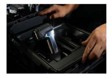
**Step 29:** Install the HVAC controls. Reconnect all connections.
