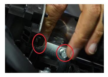
**Step 21:** You can see the 10mm bolt and the factory connector you need to disconnect. This factory connector will mate to our stowable shifter harness.
