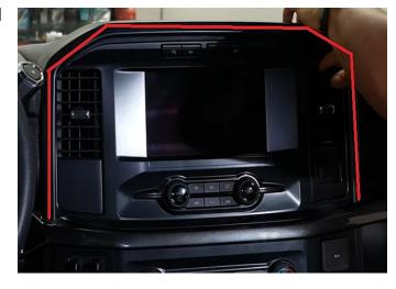
**Step 2:** Remove the trim from below the radio controls. It is only held in with retainer clips.
