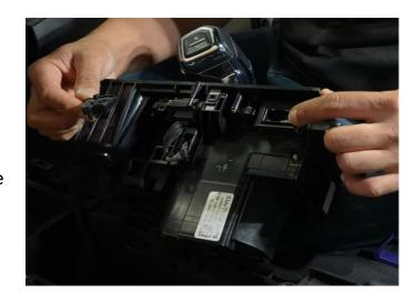
**Step 11:** Pull up on the cubby with the USB hub, it is only held in with retainer clips. You only need to move it up just enough to route the harness.
