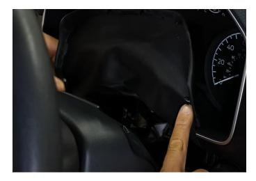
**Step 27:** Install knee bolster and secure into place with the two 7mm screws.
