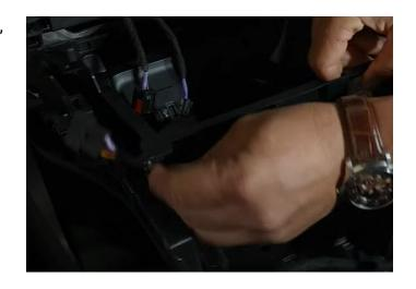
**Step 12:** You can now secure the stowable shifter into place with the three 10mm bolts.
