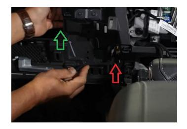
**Step 24:** Route the stowable shifter harness till you can plug it into the factory connector you disconnected earlier.
