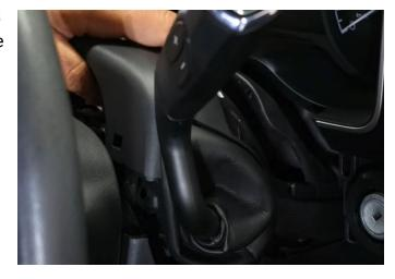
**Step 20:** Next is to remove the column shifter. Start with the two 8mm bolts. There is a single 10mm bolt on the other side holding the column shifter.
