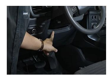
**Step 24:** Next open the bottom knee bolster panel to expose the two 7mm bolts that need to be removed. The lower panel will come free once the two bolts are removed, place it off to the side.
