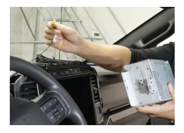
**Step 32:** Angle the ACM downward and slide it into place.
