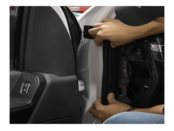
**Step 20:** Next remove the trim panel to feed cable into the dash. Use your pry tool to pull the panel off, it is only held in with retainer clips.
