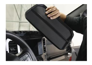
**Step 3:** You'll see the two holes where two 7mm bolts are that need to be removed.
