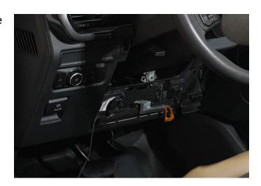
**Step 27:** Route the cable up to the ACM. This can be a pain but if you use a fish wire it can make the process much easier. We used a long zip tie with the end slightly curved. Feed it up in the dash going to the ACM.
