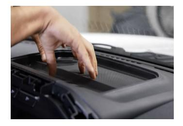
**Step 38:** Lastly reinstall the last trim panel that goes above the radio screen. You'll hear the retainer clips snap into place.
