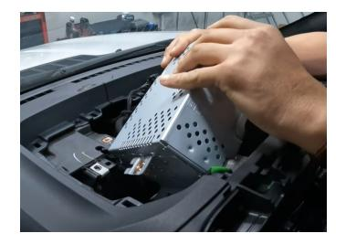
**Step 8:** Once you have the factory ACM out enough to gain access to the its rear. You'll want to disconnect all the connections at the rear of the ACM.
