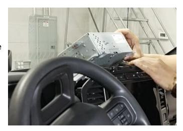
**Step 33:** You will need to reinstall the four 7mm bolts from around the ACM, two per side.
