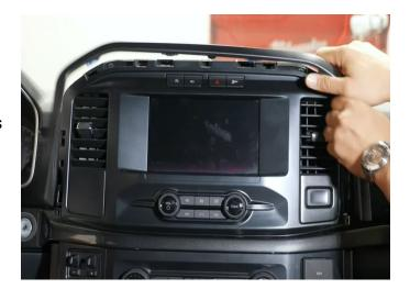
**Step 2:** Remove the rubber mat from above the screen and place it off to the side.
