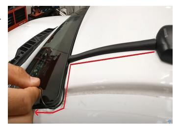
**Step 14:** You'll be able to use your pry tool or a flathead screwdriver to pull up the window's rubber strip to feed the antenna cable under it for the neat and clean finish.
