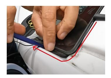
**Step 15:** Once you reach the gap between the fender and pillar, you can feed the cable through the gap into the door well.
