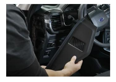
**Step 23:** We will need to remove the knee bolster to gain access to route the antenna cable up to the ACM.
