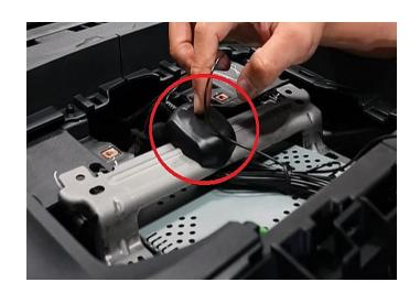
**Step 36:** Reinstall the center console cover. Remember to reconnect the one connection under it. Secure into place with the two 7mm bolts.
