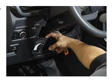
**Step 30:** You can reinstall the upper knee bolster then put the two 7mm bolts back into place for the lower knee bolster. Then close the lower knee bolster up.
