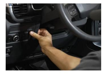
**Step 26:** You can now pull the cable up from the foot well into the opening that was behind the upper knee bolster.
