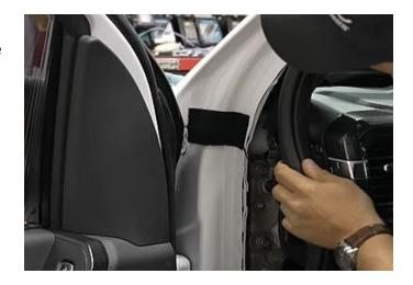
**Step 18:** Route the cable under the weather stripping, be sure to route the cable going down the strip not to pinch the cable. You can see the correct path for the cable.
