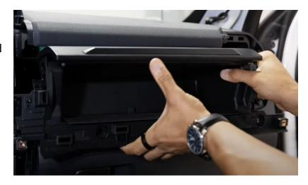
**Step 27:** Remove the two 10mm bolts holding the lower end of the air bag in place.
