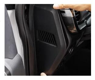
**Step 72:** Reinstall the steering wheel column cover. There are clips along the top and sides.
