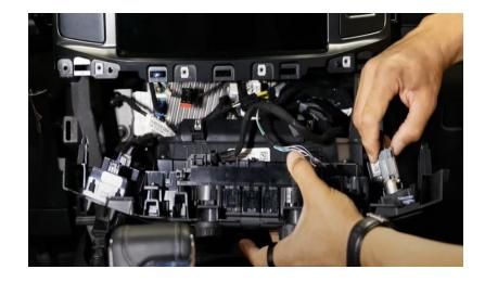
**Step 20:** Remove the three 7mm bolts from around the radio.
