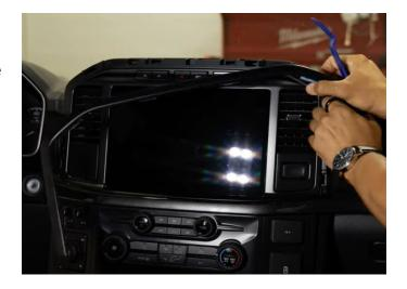
**Step 2:** Next is to remove the trim panel from below the screen. Start by the key cylinder. Use your pry tool as it is only held in with retainer clips. Place it off to the side.
