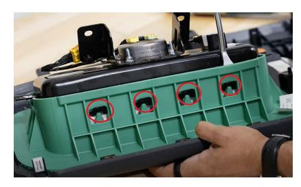
**Step 44:** Install airbag in the new passenger side dash. It is the same process in reverse.
