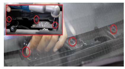
**Step 38:** Starting on the passenger side, Use your pry tool to lift on the clip to release, the rest of the passenger dash is held in with retainer clips. Firmly lift to release retainer clips. Lift to see the yellow airbag connection.
