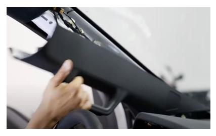
**Step 32:** Remove the trim panel from the driver's side with pry tool. It is only held in with retainer clips.
