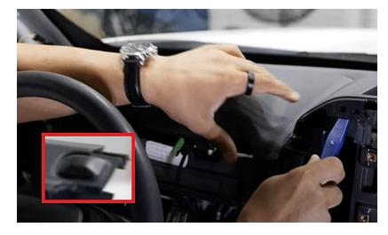
**Step 41:** Move the Sun sensor to the new driver's dash. The sun sensor is only held in with clips, squeeze to release then snap sun sensor in new driver's dash.
