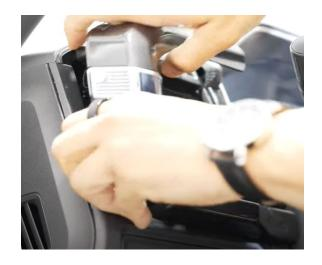
**Step 6:** Remove the one 7mm bolt from behind the trim panel you just removed.
