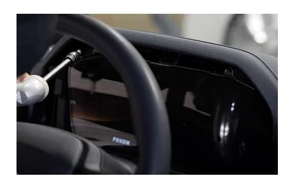
**Step 63:** Reinstall the three 7mm bolts from around the screen.
