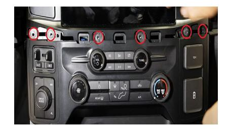
**Step 75:** Reinstall the side trim panels along the center console. Remember to slide the trim forward then inward.
