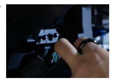
**Step 68:** Reinstall the one 7mm bolt to the right of the driver's AC vent.
