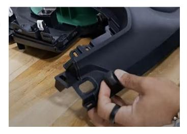
**Step 42:** Let's move the Airbag over to the new passenger side dash. First remove the four 7mm bolts on the sides of the airbag.
