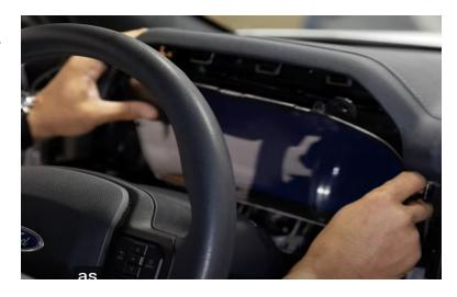
**Step 62:** Secure the new cluster into the dash with the four 7mm screws.
