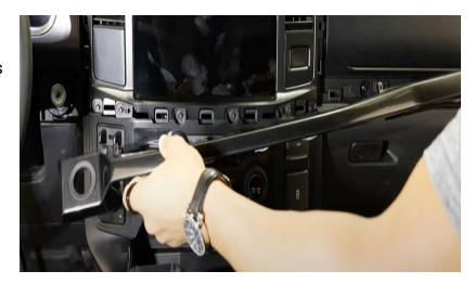
**Step 77:** Lastly reinstall the last trim panel that goes above the radio screen. You'll hear the retainer clips snap into place.
