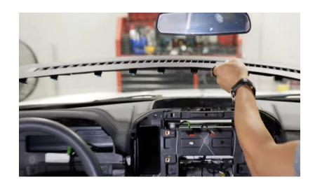
**Step 51:** Reinstall the driver's and passenger side pillars with the two 10mm bolts per side.
