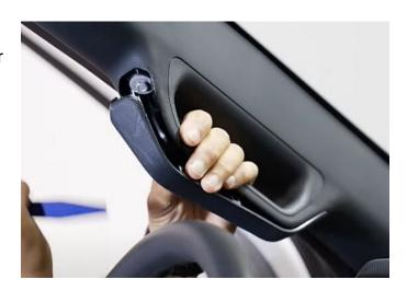
**Step 30:** Remove the two 10mm bolts.
