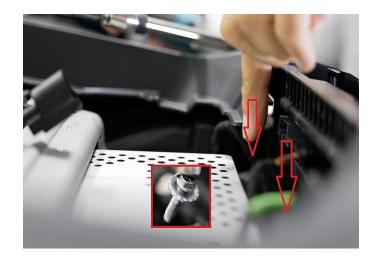
**Step 24:** You can now pull the screen out. Lean the screen forward so you can get to the rear of the screen to disconnect it. Carefully place the screen to the side.
