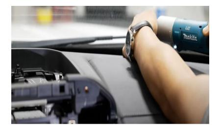
**Step 50:** Install the long shroud close to the windshield.
