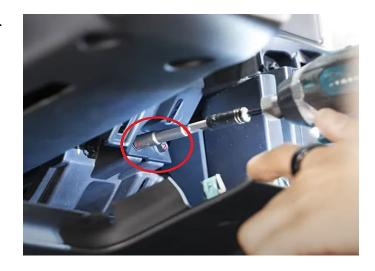
**Step 5:** Remove the trim panel below the driver's AC vent. Use your pry tool as it is only held in with retainer clips. Place it off to the side.
