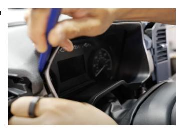
**Step 9:** Disconnect the three connections going to the key cylinder and place the cluster bezel off to the side.
