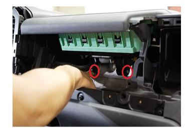
**Step 53:** Reinstall the three T20 Torx screws under the passenger side dash lip.
