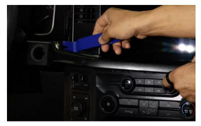
**Step 3:** Pull below the key cylinder to pop out two retainer clips to expose two 7mm bolts that need to be removed. You do not need to remove the knee bolster fully.
