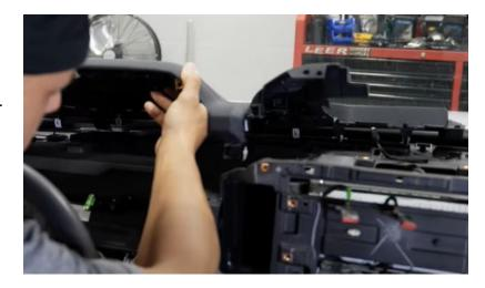
**Step 48:** Install the new passenger side dash with the airbag you transferred over.
