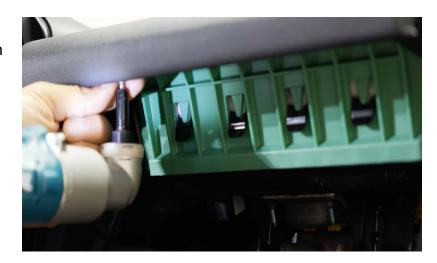
**Step 54:** Reinstall the glove box the secure with the three T25 Torx screws.
