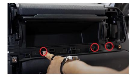
**Step 26:** Pull the glove box straight back as there are still some retainer clips holding it in place. Once removed place off to the side.
