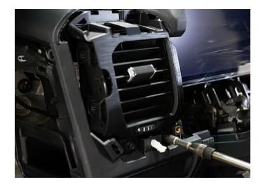
**Step 65:** Next is the cluster bezel, reconnect the key cylinder connections.
