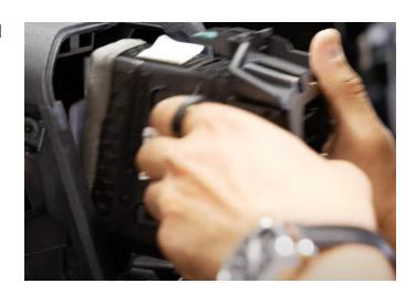
**Step 36:** Remove the dash shroud that is up against the front windshield. It is only held in with retainer clips. Use your pry tool to life on the left or right side to start releasing the retainer clips. Place it off to the side.
