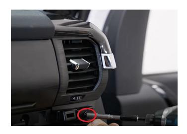
**Step 15:** Remove the side trim panel. You'll see the green retainer clips once the AC vent was removed.
