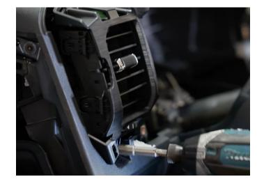
**Step 35:** The driver's AC vent can now be pulled out. It is only held in with retainer clips.
