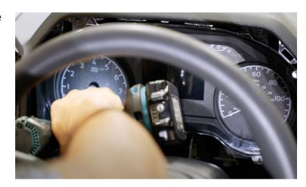
**Step 11:** Now the real fun begins. If you haven't already, disconnect your battery as we will be working with the passenger airbag. Once that is done, we need to remove the passenger pillar. Start by removing the cap with a pry tool.
