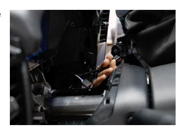
**Step 66:** Install the new cluster bezel around the new full digital cluster. You'll hear the retainer clips snap into place.
