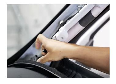
**Step 14:** Remove the 7mm bolt below the passenger side AC vent then pull the AC vent out as it is only held in with retainer clips.
