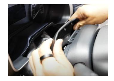
**Step 8:** Using your pry tool, remove the trim from around the factory cluster.
