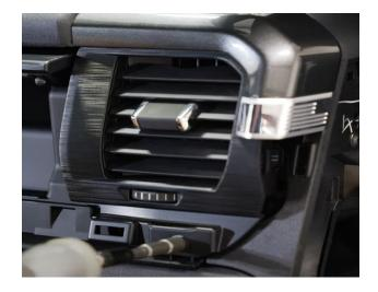
**Step 56:** Reinstall passenger side trim panel. It just snaps into place.
