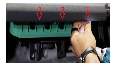
**Step 29:** Going over to the driver's side. Time to remove the driver's side pillar. Remove the cover with your pry tool.
