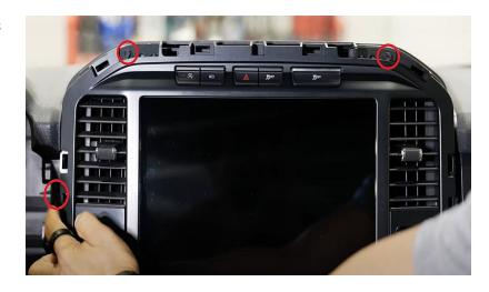
**Step 21:** Next remove the rubber mat from above the radio screen to expose the two 7mm bolts needed to be removed to get to the two 7mm hidden bolts.
