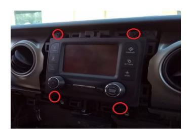
**Step 6:** Lean the factory radio toward yourself, do not pull too hard. You'll see the factory fakra connections, USB connection, and the 52 black connector. Disconnect these connections. Place factory radio off to the side.
