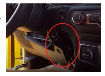
**Step 2:** Use your pry tool to pop out the HVAC controls from the right side. Either disconnect the connections then place it to the side or carefully let the controls hang while you finish installing the radio. The HVAC controls are only held in with retainer clips.
