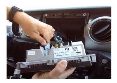
**Step 9:** Push radio into place, make sure not to pinch any wires. Secure radio with the four 7mm screws you removed earlier.
