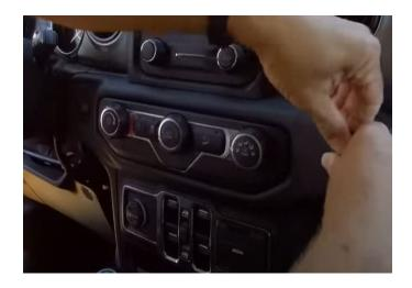
**Step 3:** There are two 7mm screws holding the factory bezel around the factory radio. Remove these two screws.
