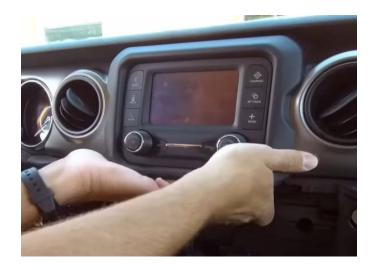
**Step 5:** You now have access to the four 7mm screws holding the factory radio in place. Remove all four screws.
