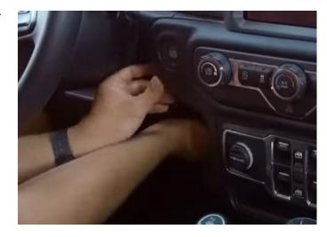
**Step 14:** Start the vehicle to see the new radio power on. If it doesn't double check your connections and your radio fuse, which is an inline fuse going from the battery to the firewall.
