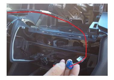
**Step 14:** You'll see the factory LVDS cable plugged into the APIM. Disconnect the cable and plug in our LVDS cable into the APIM.
