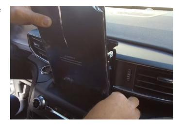
**Step 26:** Reinstall the three 8mm bolts behind the screen.
