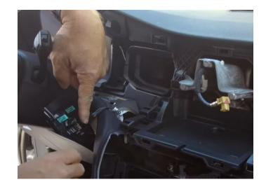
**Step 11:** Pull up on the trim panel on the opposite side of push to start button. You do not need to remove the trim fully, you just need it out of the way enough.
