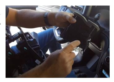
**Step 6:** Next remove the liner from below the screen. Place it off to the side.
