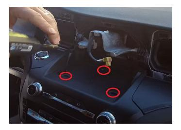
**Step 8:** Remove the climate controls, they are only held in with retainer clips. With a good pull the climate controls will be released from the dash.
