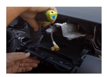
**Step 18:** Now that the tray is installed and secure. Snap the trim panel with the push to start button back into place.
