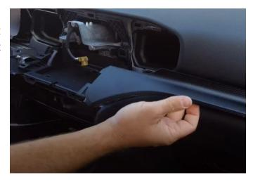
**Step 12:** Remove the trim panel below where the factory screen was installed. It is only held in with retainer clips.
