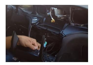
**Step 21:** To reinstall the climate controls, you need to angle the top plastic hooks so the climate controls install properly. You'll hear the retainer clips snap back into place.
