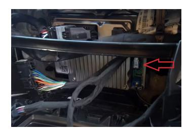
**Step 15:** You can remove the factory LVDS cable from the screen bracket then tuck it away in the dash. You can push the plastic clip on our LVDS cable into the same spot you just removed the factory LVDS cable from.
