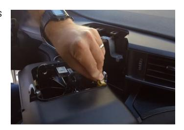
**Step 24:** Route the LVDS cable the same way we did so it doesn't get pinched. There are three slots and two retainer clips to hold the screen in place.
