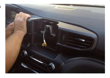
**Step 23:** Screen install time! Take the new LVDS cable and plug it into the rear of the 10" screen.
