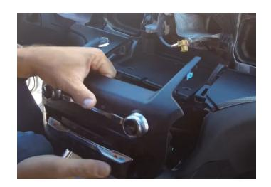
**Step 9:** Disconnect the climate controls. There are four connections that need to be released.
