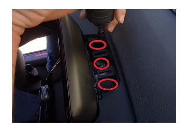
**Step 3:** You can now pull the 8.4" screen out of the dash, disconnect the factory LVDS cable then set screen off to the side.
