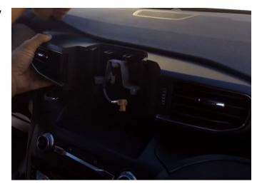
**Step 5:** Once you have the factory vent trim out. Remove the factory vents and swap them to our vent bezel in the kit. There are four, two per side, clips holding the vents in place.
