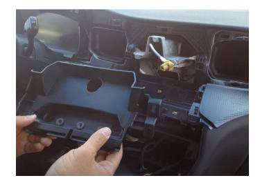
**Step 17:** Once the new tray is snapped into place, you can reinstall the three 7mm screws you removed earlier.
