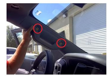
**Step 35:** Now you can install the new rear view mirror into place. The new mirror will slide down into place, in the same spot as the old factory mirror.
