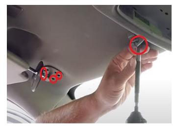
**Step 5:** Remove the rear pillar covers, they're only held in place with retainer clips. Slide them down so they are out of the way.
