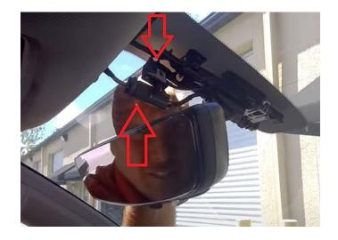
**Step 38:** Tuck the wires away above the head liner and put the two connectors on either side of the mirror.
