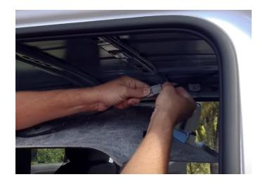
**Step 15:** Time to remove the 12 screws holding the rear third brake light fixture in place. All four bolts and eight nuts are 10mm.
