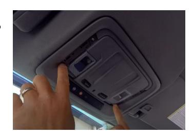
**Step 45:** Now that the two screws are in place. put the center light fixture trim covers back into place. They will just snap into place.
