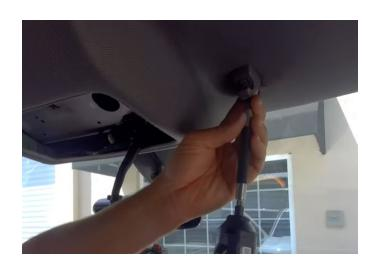
**Step 42:** Now for the sun visor, secure back into place with its three screws.
