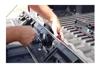
**Step 21:** Secure the new third brake light into place with the four T20 screws.
