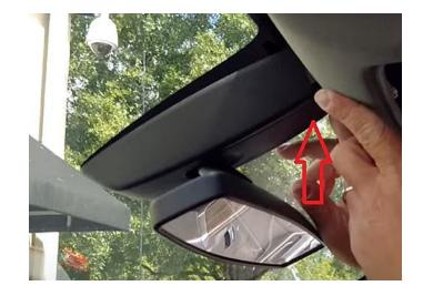
**Step 8:** After which the plastic shroud will slide down. Place it off to the side.
