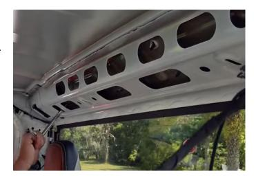
**Step 27:** Push the headliner back into place, the center light fixture once snapped in will help hold the liner in place while you secure the hooks. There are two push pin connectors at the rear of the liner, snap these into place.
