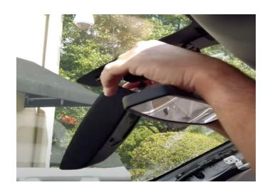
**Step 9:** There is only one screw holding the mirror in place. Remove it and place the mirror off to the side.
