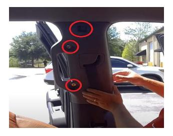
**Step 32:** You should have the wire you routed to the front hanging down from the upper center light fixture.
