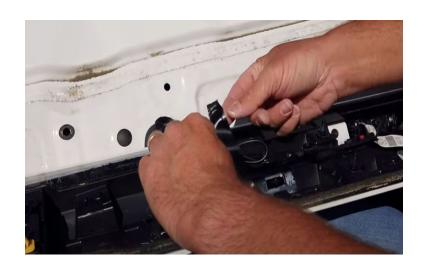
**Step 24:** Flip the third brake light fixture around and snap it into place.
