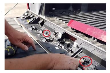
**Step 20:** You can slide the new third brake light into place. Feed the cable through the factory hole.
