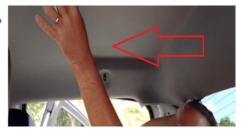
**Step 14:** To help free the head liner, there are some wire clips in the front of the vehicle you can disconnect, also disconnect the connector at the rear of the head liner.
