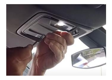
**Step 2:** Remove the two screws from under the plastic covers.
