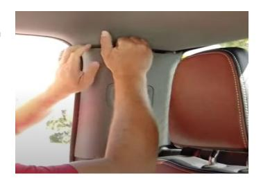
**Step 6:** Remove the coat hangers from the rear head liner. Using the Flathead, pull the plastic tab back which exposes the screw to remove.
