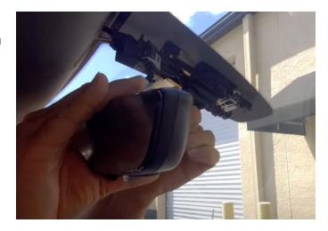
**Step 36:** Hand tighten the torx screw into place to hold the new rear view mirror in place.
