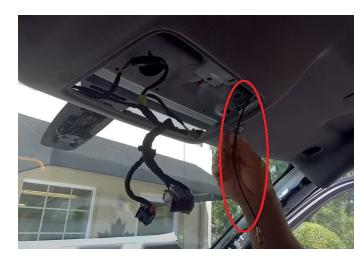
**Step 33:** You can now plug in the two connections to the mirror and test. Once in reverse you'll see the camera on the rear view mirror.
