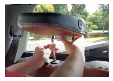
**Step 12:** Now only holding the head liner in place is the door seals which release the head liner if you just pull the head liner down, also the center light fixture for the rear seats. If it is only held in with retainer clips, pull it down to release the light fixture.
