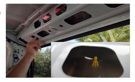
**Step 17:** Lean the rear third brake light fixture down then remove the factory wiring. Disconnect the plastic clips and third brake light connector. Pull the red tab back to release the lock.
