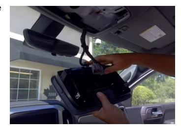
**Step 44:** Secure center light fixture into place with its retainer clips. Then secure with the two screws you removed earlier.
