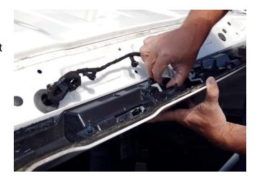
**Step 18:** Now to remove the third brake light from the third brake light fixture or spoiler. There are four T20 screws to remove.
