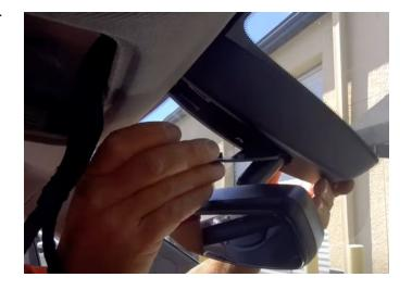
**Step 41:** Time to reinstall the sun visors. Start with the visor clips. Secure into place with the one screw.
