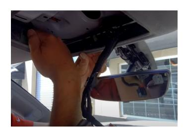
**Step 39:** Reinstall the mirror cover, slide it into place from the bottom of the rear view mirror. The tabs need to lock into place. Be careful not to break the tabs.
