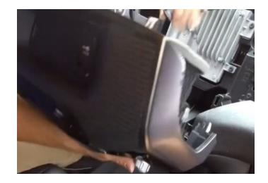
**Step 14:** Push the bezel/screen into place. It is held in with retainer clips that you should hear snap back into place.
