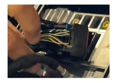
**Step 5:** Remove your factory radio module if you had a 8.4" UAV from factory by removing the four T10 screws. If you had a 8.4" UAQ or other all in one unit radio then remove it be unscrewing the same four T10 screws.
