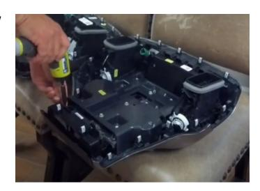
**Step 12:** You can now take the Bezel/Screen and start making the connections. Use our UAX harness to plug into the screen and use our LVDS cable to plug into the screen.
