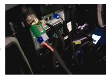
**Step 3:** Lean Bezel/Radio forward so you can start disconnecting the harnesses attached to its rear.
