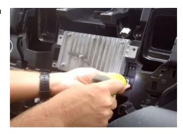
**Step 6:** For the UAV, once the module is loose you can lean it forward and disconnect all the connections at its rear. Place the module off to the side.
