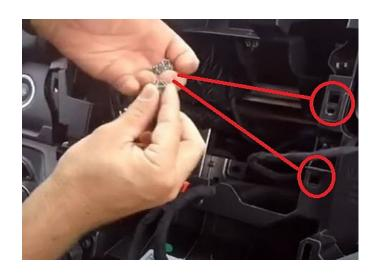
**Step 9:** Mount the new UAX module with the four T10 screws.
