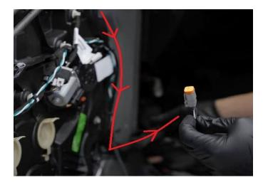
**Step 56:** Once you get to the sleeve the door hook was attached to. You can either feed the mirror harness through the sleeve or zip tie the mirror harness to the back side of the sleeve.
