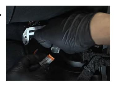
**Step 66:** Push the harnesses behind the kick panel, reconnect the factory white lever connector, reattach it to kick panel then cover it back up.
