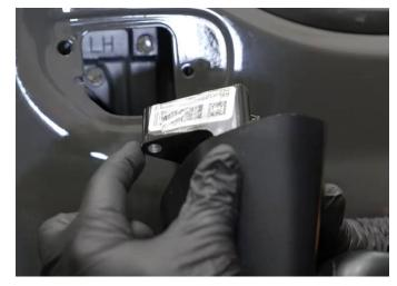
**Step 48:** Going back to the inner door, remove the upper right grommet. Be careful not to pull the factory mirror harness out of the door as there is no mirror connected to it at the moment.
