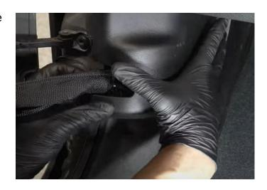
**Step 69:** Install the Security Gateway Module Bypass in the appropriate place. Then proceed with genie programming. This step is only needed for 2018+ vehicles. To find your vehicle's bypass location click the link: <u>OBD Genie Bypass</u>
