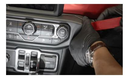
**Step 32:** Remove the one philipshead screw from above the window controls.
