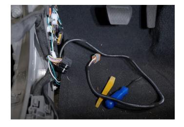
**Step 26:** Next we need the mirror jumper harness. Plug it into the body harness.
