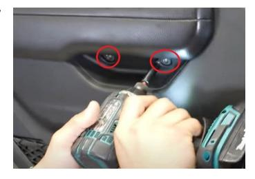
**Step 41:** At the bottom of the door panel, there are two T20 screws to be removed.
