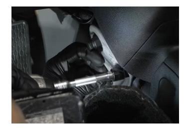
**Step 68:** Reinstall the driver's side kick panel the same as the passenger side.
