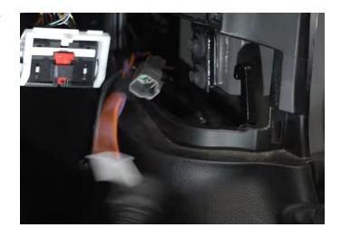
**Step 65:** Reinstall the 10mm screw, re-hook the wiring sleeve then plug in the mirror harness into the body harness.
