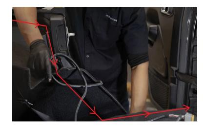
**Step 23:** Feed the body harness past the driver's seat. Routing the cable under the trim panels.
