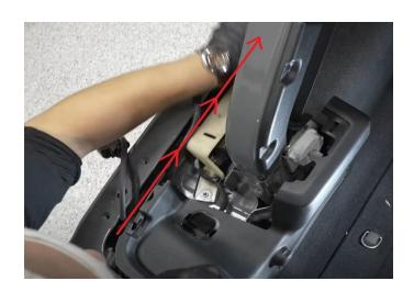
**Step 18:** Feed the body harness behind the trim panel till you get to this point. Reinstall the trim panels you just removed from the rear of the vehicle.
