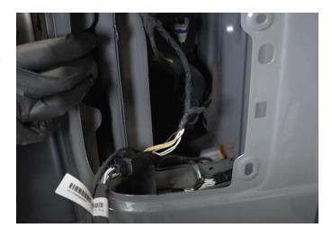
**Step 9:** Once the taillight harness has been run, you can install the new passenger side taillight.
