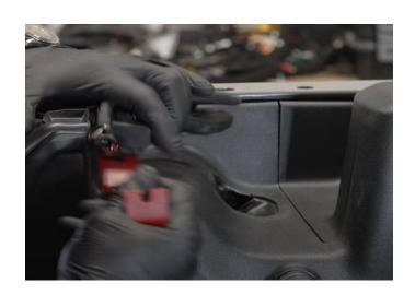
**Step 12:** Pull the weather stripping back and use your pry tool to free the retainer clips holding the trim panel in place. You don't need to remove the panel fully, just enough to get to the under side of the top of the panel. This is where a rubber grommet is located to feed the taillight harness through.
