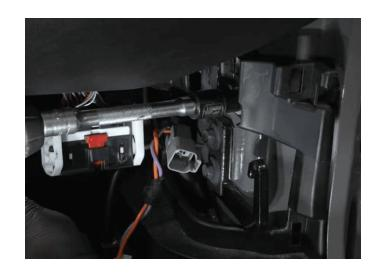
**Step 63:** Zip tie the mirror harness to the factory wiring behind the kick panel you just removed.
