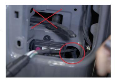
**Step 6:** From under the vehicle. Follow the factory wiring harness till you get to the driver's side taillight. Zip tie along the factory wiring harness.
