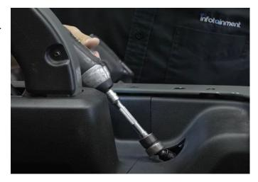
**Step 3:** You should be able to slide the factory taillight out. Disconnect the taillight by pushing the red locking tab up to release the connection.
