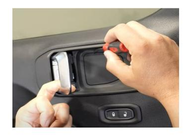
**Step 39:** Remove the T30 screw from behind the internal door handle.
