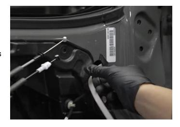
**Step 50:** Taking our mirror harness, plug in the factory mirror connection into our mirror harness. Next grab the zip tie or what you used and attach the gray connector from our mirror harness and feed it down into the door cavity.
