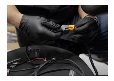
**Step 27:** Next we will be running the mirror jumper harness passenger side connector to the passenger side.
