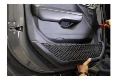
**Step 44:** Disconnect the main door harness from the door panel. Pull the red locking tab up to unlock then pull connector apart to release.
