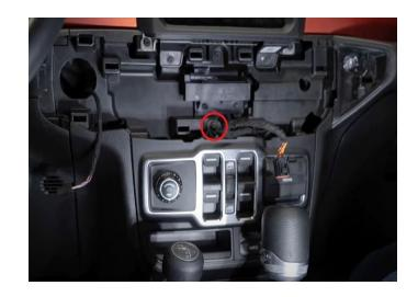
**Step 33:** Pull the rest of the panel out as it is only held in with retainer clips now. This will give you access to the 12 volt outlet connector.
