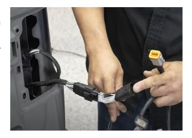
**Step 5:** Feed the taillight harness into the lower right opening. Do not put it through the top left hole as this is used by the swing gate arm. Zip tie the taillight harness to factory wiring for neat and clean finish.
