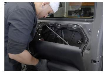
**Step 59:** Using your pry tool, pop the cover of the foot well panel.
