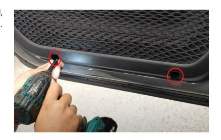
**Step 42:** This step is optional but we like to remove the door hook that holds the door wiring. This again isn't necessary but it makes things easier so it's recommended. There are two T20 screws holding the hook in place.
