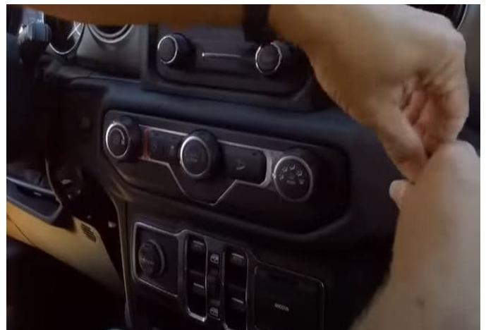
**Step 3:** There are two 7mm screws holding the factory bezel around the factory radio. Remove these two screws.
