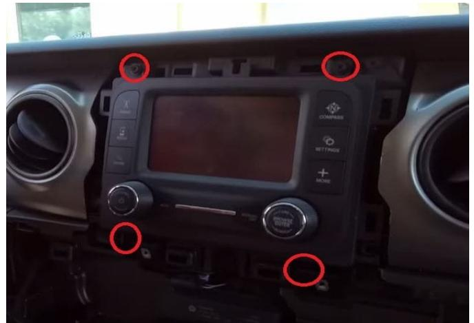
**Step 6:** Lean the factory radio toward yourself, do not pull too hard. You'll see the factory fakra connections, USB connection, and the 52 black connector. Disconnect these connections. Place factory radio off to the side.
