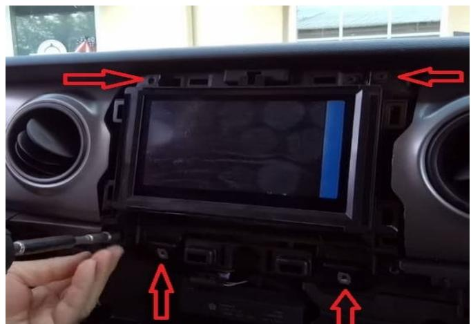
**Step 10:** Snap new bezel into place. This bezel has angled corners while your factory bezel has rounded corners. This is why you need a new bezel.
