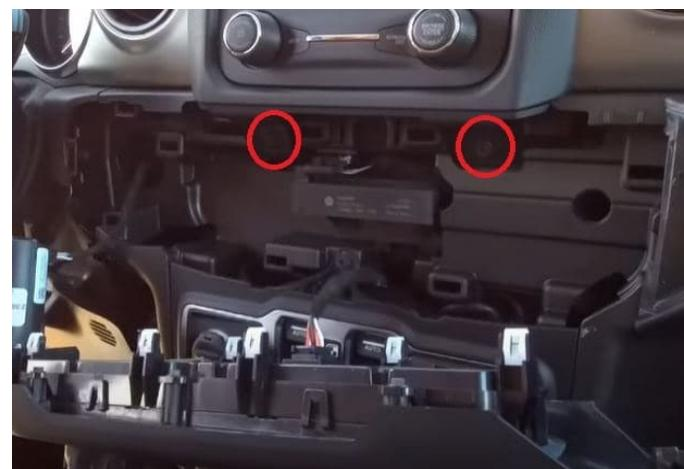
**Step 4:** You can now pull the factory bezel out and place it to the side. The rest of the bezel is only held in with retainer clips.
