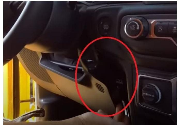
**Step 2:** Use your pry tool to pop out the HVAC controls from the right side. Either disconnect the connections then place it to the side or carefully let the controls hang while you finish installing the radio. The HVAC controls are only held in with retainer clips.
