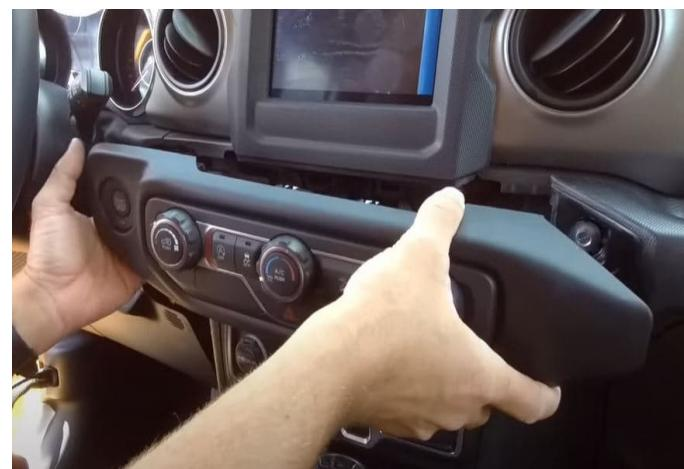
**Step 13:** Push the top corner of the knee bolster back into place. You'll hear the retainer clips engage.
