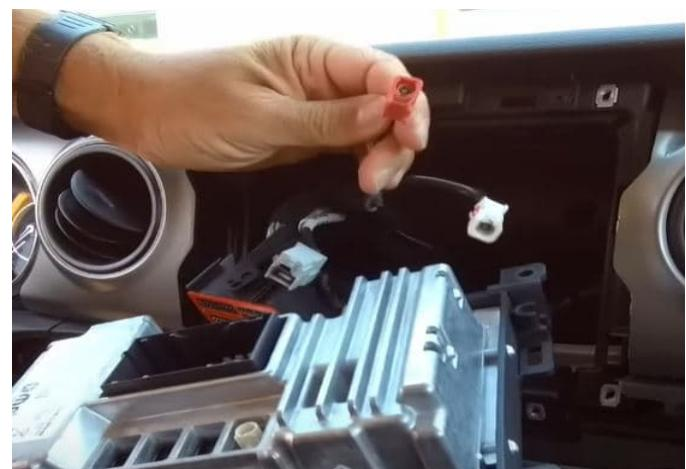
**Step 7:** For the UAG, you will need an antenna for XM signal. You can either use a new antenna that does both signals or a stand along XM antenna.
