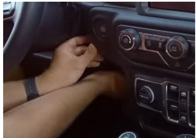
**Step 14:** Start the vehicle to see the new radio power on. If it doesn't double check your connections and your radio fuse, which is an inline fuse going from the battery to the firewall.
