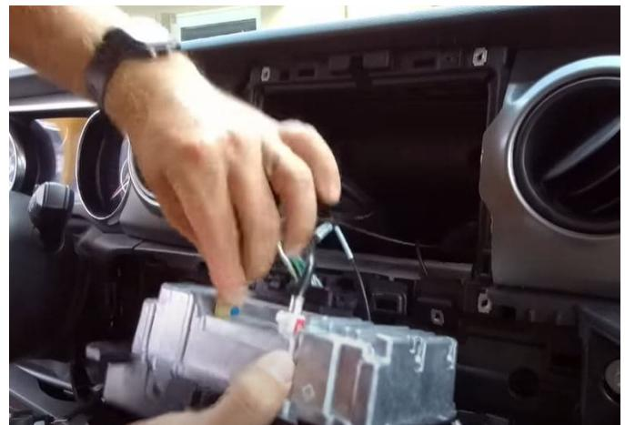
**Step 9:** Push radio into place, make sure not to pinch any wires. Secure radio with the four 7mm screws you removed earlier.
