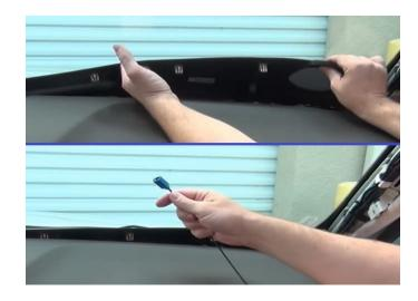
Step 11: As you feed the blue fakra down the cavity, you'll need to reach under the glove box location till you feel the blue fakra cable. Pull the cable through and mount the GPS antenna under the dash with either some double-sided tape or some zip ties. Just remember to have no metal above the GPS antenna. It is always a safe bet to test location signal strength before permanently mounting antenna.
