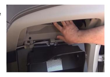
**Step 3:** The factory HMI can be hard to see as the cables cover it. Disconnect all five connections.
