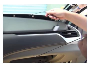
**Step 12:** Plug in the blue fakra from the GPS antenna into the blue fakra on the far left side of the new HMI module. You'll hear it clip and lock into place. Zip tie any excess cable out of the way for neat and clean finish.
