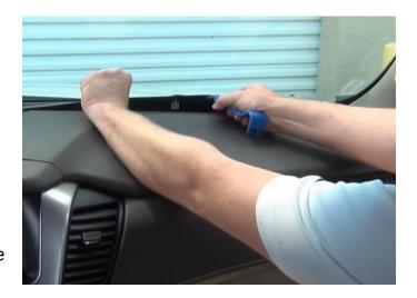
**Step 8:** Next remove the two plastic covers along the passenger pillar using a pry tool to expose the two 10mm screws holding the pillar in place.
