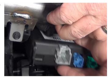
**Step 5:** Slide the new HMI module in the space for the factory HMI and reconnect the five connectors in the same spots as the factory connections.
