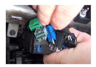
**Step 6:** Once the new HMI is installed, you'll see the blue fakra antenna connection left unpopulated. This is where the GPS antenna plugs into.
