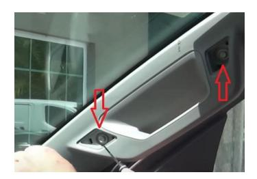
**Step 9:** Remove the two 10mm screws then place pillar off to the side.
