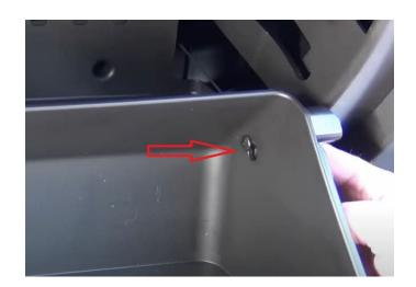
**Step 3:** Next let the glove box hang down so you can remove the four T15 Torx screws. Once the screws are removed the glove box will come free, place it off to the side.
