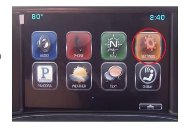
**Step 15:** You'll see the new "Nav" icon on the radio, hit it to see the map. GPS should pick up your signal right away but if it doesn't drive around for a day for the GPS antenna to get enough satellites to get good navigation tracking.
