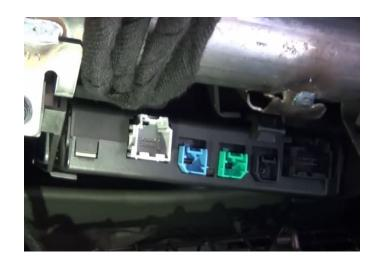
**Step 6:** Slide the new HMI into the factory spot then connect all the connections the same as it was for the factory HMI.
