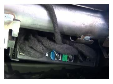
**Step 5:** Disconnect all the connections on the factory HMI. The factory HMI should slide out with a bit of wiggling.
