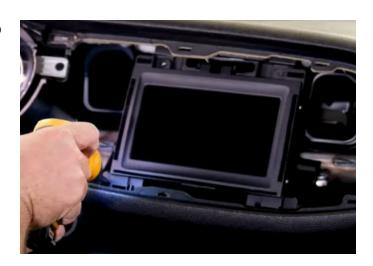
**Step 9:** Take the bezel and carefully mount it back into place. You may need to give it a good smack with the palm of your hand to engage the retainer clips.
