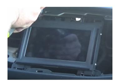
**Step 3:** Disconnect all the connections on the rear of the factory radio. Set the factory radio to the side.
