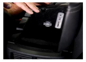
**Step 11:** The USB hub is held in with retaining clips, four total. You'll need to pry up the USB hub and using a pick or flathead screwdriver to depress the retainer clips to release the factory USB hub.
