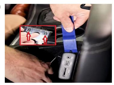
**Step 12:** Once you have the factory USB Hub removed, disconnect the two connections on its rear. Depress the locking tabs to get the connections to release.
