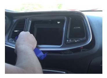
**Step 2:** Remove the four screws from around the stock radio. These will be 10mm bolts or Philip screws.
