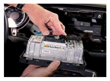
**Step 8:** Place the radio into the dash and line up the mounting holes. Reinstall the four 10mm bolts or the four screws to hold the radio in place.
