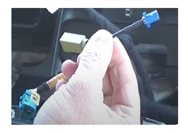
**Step 6:** If you need to install a new XM and/or GPS antenna, you'll just plug the fakra into the yellow/curry port on the rear of the radio then route the antenna under the dash. As long as there is no metal above the antenna, then it should get a good signal. If not, then move antenna and test till you find a good spot.
