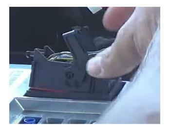
**Step 5:** Some vehicles will not have an XM or GPS antenna as the factory radio didn't call for the antennas installation. In these case you'll need to install a new antenna to get those signals but if you have said antenna from factory then use the fakra conversion cable in the kit to plug the antenna into the yellow/curry fakra port on the rear of the radio.
