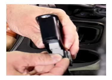
**Step 14:** Push the new USB hub into place. Its retainer clips will engage to hold the USB hub in place.
