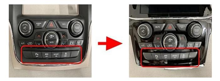
**Step 1:** Find a clean & soft surface to lay your Jeep's factory radio bezel face down. Locate the black plastic housing on the lower portion of the radio bezel. Remove ten Torx T8 screws (Six around the perimeter and four in the center). Pull off the climate control housing.
