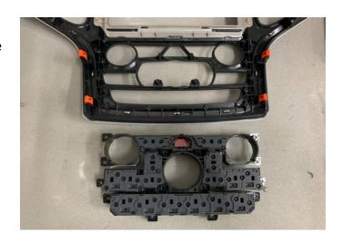
**Step 5:** Install the middle component on the UAQ radio bezel first. Insert it at an angle to allow the bottom portion to tuck behind the lower screw holes.
