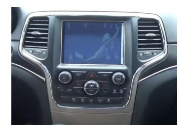
**Bezel Button Swap:** The bottom row of controls on the bezel may not match your factory bezel. If they do not match, you'll need to swap the controls from the old bezel over to the new bezel. Instructions below.
