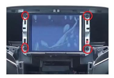
**Step 15:** Reattach the bezel's HVAC control connector and install bezel back into place. Push firmly to get retainer clips to lock into place.
