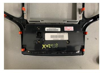
Step 2: Remove eight Torx T8 screws around the
