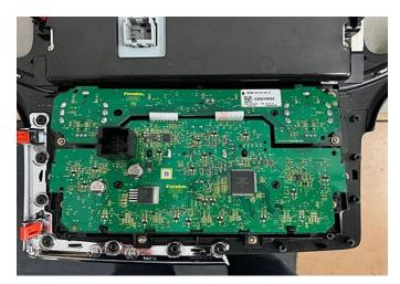
**Step 8:** Place the climate control housing over the circuit boards. You may have to slightly bend the bezel a tad to get the housing to secure into place. Install the remaining ten Torx T8 screws. Done!
