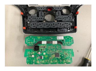
**Step 4:** Remove four Torx T8 screws. Then pull away the three remaining components from the radio bezel.
