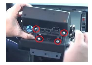
**Step 8:** Once new USB hub is installed you can reinstall the cubby with the four screws.
