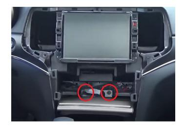
**Step 6:** Put your emergency brake on and put the vehicle into neutral. This will give you enough room to get the cubby out so you can disconnect the factory USB hub.
