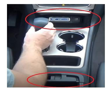
**Step 2:** The cup holder and gear shifter panel are only held in with retainer clips. You can pull up from the front most part to release the clips.
