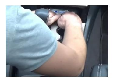
**Step 3:** With the panel unclipped into place you can turn it to get access to the two 7mm screws.
