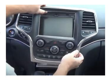
**Step 5:** Now with the radio bezel out of the way you gain access to two more 7mm screws to remove.
