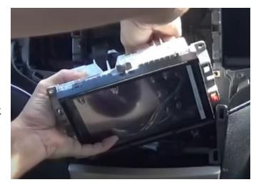
**Step 14:** Push the radio back into place and secure it with the four 7mm screws.
