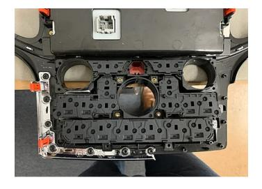
**Step 7:** Install the two circuit boards and snap into place. Install eight Torx T8 screws around the perimeter.
