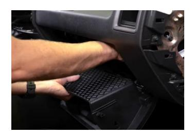
**Step 22:** Reinstall the trim panel on the passenger side.
