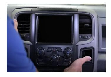
**Step 27:** Reinstall the two T20 screws above the radio.
