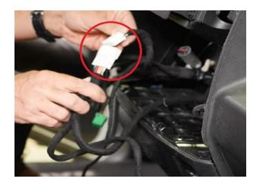
**Step 24:** Let's install the RA3/RA4 radio. Connect all the factory connections that went to the old radio. White fakra for AM/FM, Yellow fakra for GPS/XM antenna, Red fakra for digital backup camera for newer vehicles, gray USB hub connection, and the 52 pin black connector for all other signals.
