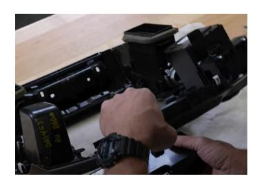
**Step 9:** Next lets install the HVAC module. Start by removing the trim panel on the passenger side with your pry tool. It is only held in with retainer clips.
