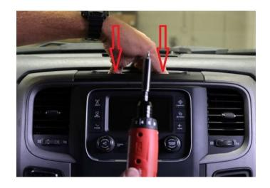
**Step 3:** The rest of the factory bezel are only held in with retainer clips. Using your pry tool or flathead screwdriver to pry the factory bezel up.
