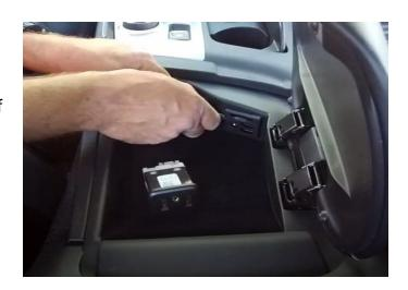
**Step 9:** Once you have the factory USB hub removed. Take the new USB hub and plug in the two factory connections to the rear of the USB hub.
