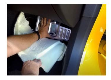
**Step 5:** Move the bracket off to the side, behind it you'll see the vehicle's BCM. There is a tab on its right you can push in to release the BCM.
