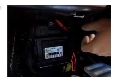
**Step 6:** With the BCM out of the way. Behind the plastic bracket, is where the factory ACM is located. With some work you can get the ACM to come free, disconnect the ACM connections.
