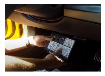
Step 3: When installing the HMI module. You'll notice if you upgraded to the IO6 with built in Navigation that there is a new blue fakra connector on the far left. This is where the GPS antenna plugs into. Reconnect your factory GPS antenna or plug in the new GPS antenna and route the antenna under the dash. Make sure no metal is above the antenna and it will get good singal.
