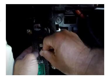
**Step 8:** Last part is to install the new USB hub into the armrest. Using a pry tool or flathead screwdriver push the side of the factoru USB hub in as tehre are plastic clips on either side of the hub.
