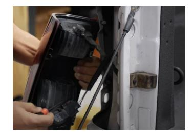
**Step 5:** Take the appropriate taillight harness and plug in the two factory connections into the LED taillight harness. The brown connection will go to the new LED taillights.
