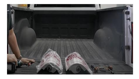
**Step 2:** Remove the two T25 Torx screws holding the factory taillights in place.
