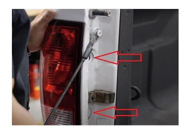
**Step 3:** Carefully remove the factory taillights. They should slide out once the two screws are removed.
