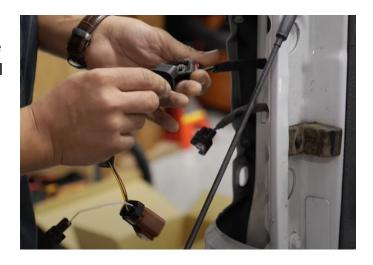
**Step 6:** Take the appropriate taillight and connect the brown connector to the rear of the taillight. Push in the red locking tab once connected.
