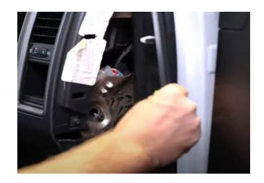
**Step 23:** Connect the HVAC harness to the factory wiring that went to the old factory bezel.
