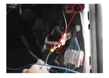
**Step 18:** Last blue wire with the big metal pin goes into the gray connector. You'll be depinning the factory wire and installing our pin in its place.
