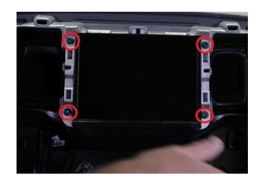
**Step 26:** Reinstall the bezel, reconnect all connections plus the new connector for the bezel. Push the bezel into place till you hear the retainer clips engage.
