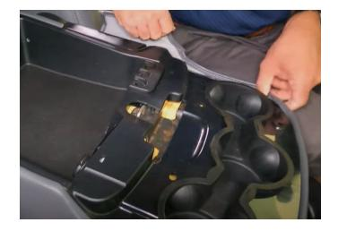
**Step 31:** You can now lift the cup holder up to get your hand under it toward the rear of the factory USB hub. From there you can squeeze the plastic tabs to free the factory USB hub.
