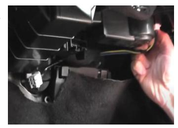
**Step 18:** Other end of the resistor harness has three connections, the white molex connection plugs into the HVAC harness, close to the HVAC module.
