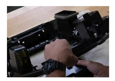
**Step 9:** Next lets install the HVAC module, this can be a 7 speed module or 4 speed, depending on what was ordered. Start by removing the trim panel on the passenger side with your pry tool. It is only held in with retainer clips.
