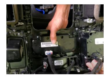
**Step 5:** To remove the factory radio, there are four 7mm screws that need to be removed.
