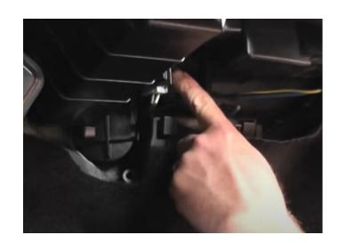
**Step 15:** There are two philips head screws holding the factory resistor in place. Remove the two screws and remove the resistor.
