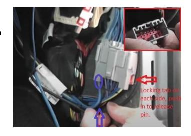
**Step 20:** Once our Pin is in place, reconnect the gray connection, push the push tab back into place.
