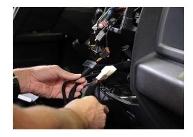
**Step 14:** Typically only heavy duty trucks need new resistor and resistor harness. Under the glove box you'll find the factory resistor to replace. Disconnect its connection.
