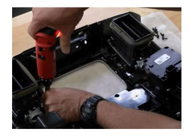
**Step 8:** Slide the new 8.4" bezel into place and secure it with the thirteen philipshead screws.
