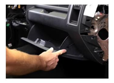
**Step 11:** You'll see two openings for the two screws on the HVAC module to slide into from the glove box side. Both screws are philipshead.
