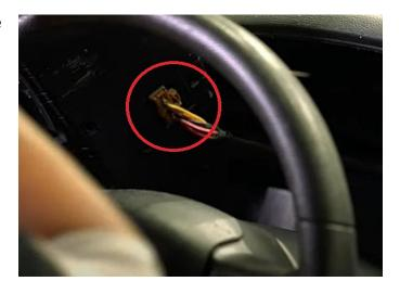
**Step 8:** Time to install the new cluster. Start by plugging it into the cluster connector.
