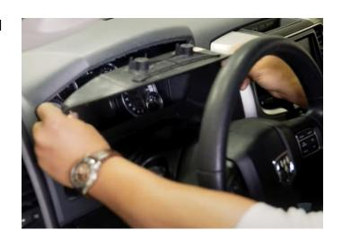
**Step 12:** Put the four 7mm screws back into the top of the cluster bezel.
