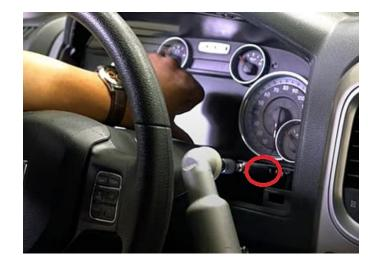
**Step 11:** Slide cluster bezel back into place and snap the retainer clips into position.
