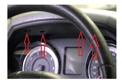
**Step 2:** Use a pry tool to get the cluster bezel loose, it is only held in with retainer clips after the four screws are removed.
