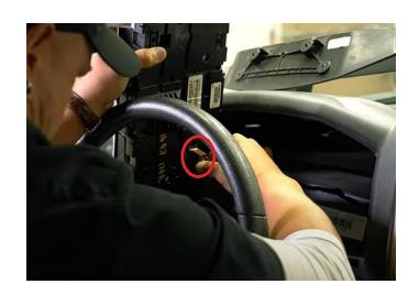
**Step 9:** Put the cluster at an angle and slide it into place.
