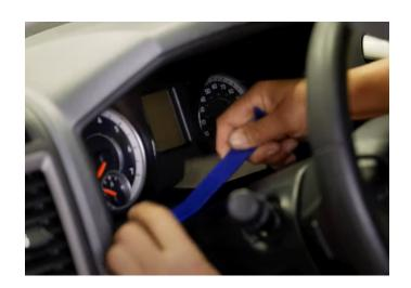
**Step 3:** Once the retainer clips have been disengaged, push down on the top of the cluster bezel to free it then place it to the side.
