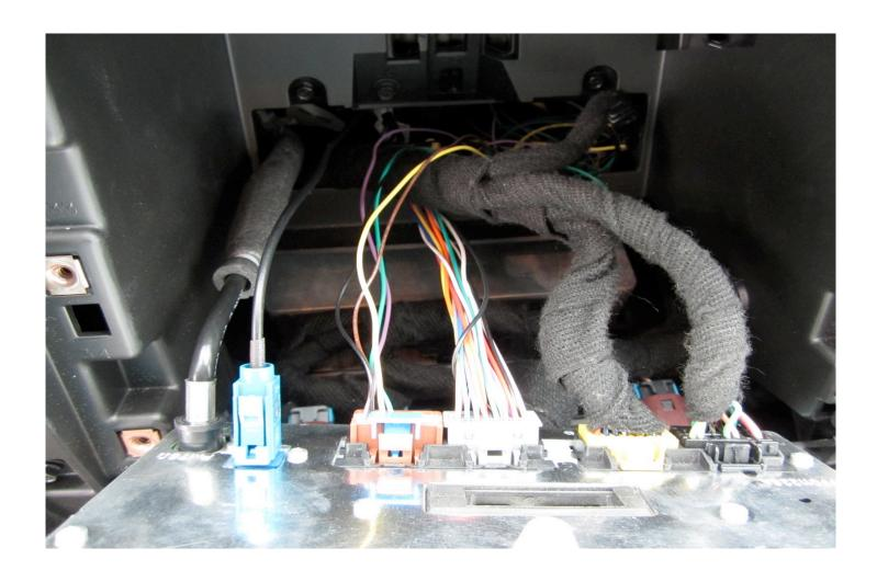
Connect all of the cables into the back of the navigation unit. This would also include the GPS antenna and FM antenna.
