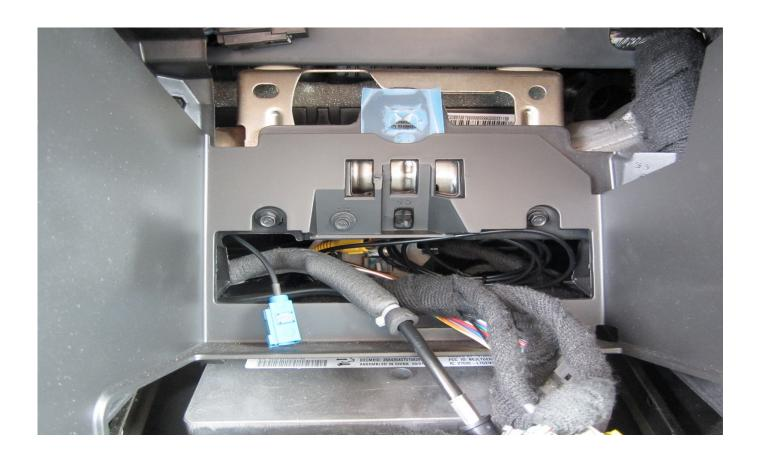
After antenna placement, feed the antenna cable down to the hole where the radio was. Make sure that the connector is fed through the lower left portion of the hole as shown in the picture above. When connecting the antenna to the back of the navigation unit, please push hard to verify a good connection.
