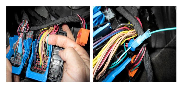
This is the vehicle speed sensor wire. The green wire from the VSS Kit brown connector has to be spliced into that green and white striped wire.
