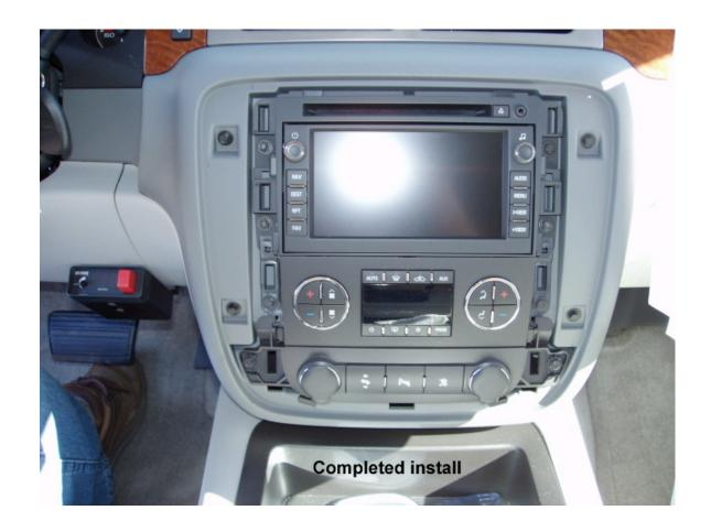
Slide the navigation unit in along with the AC controls & lighter panel. Reinstall all 8 (7mm) bolts. Reinstall the bezel/trim panel.
