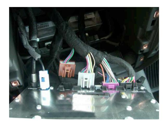
Connect the brown connector into the back of the navigation unit (connector # 4) along with the other connectors. Remember, some vehicles don't have all 4 connectors.
