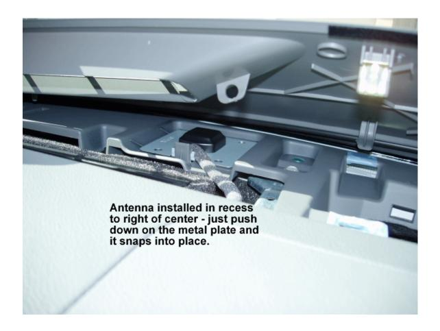
Place the antenna in the recessed area just to the right of the center. The metal portion of the antenna will fit into the plastic slot towards the windshield side and then just snap into place. Route the cable down the hole just to the right front of the recessed area as shown in the picture. Be careful not to severely bend the cable since the internal wire can break. Also, keep in mind that window tint can interfere with GPS satellite reception.
