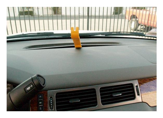
Using a plastic trim tool or a screwdriver, pry up the top dash panel as much as possible to install the GPS antenna module.
