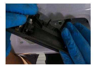
**Step 5:** Take the factory tailgate handle and new camera tailgate handle so you can swap the lock to the new handle. There are two 8mm bolts holding the lock in place. Disconnect the camera harness is attached for next step.
