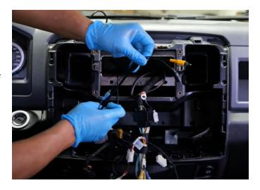
**Step 32:** Using your fingers, push the 12v outlet toward yourself to pop it free. You can then disconnect the 12v outlet and put our EZDC harness in between the factory connector for the 12v outlet and the 12v outlet.
