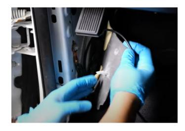
**Step 23:** Continue to route the tailgate body harness toward the center console. Zip tie along the way for the neat and clean finish.
