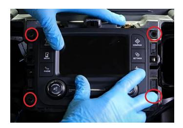
**Step 36:** Install bezel back into place, remember to make all your connections and to zip tie along the way so not to pinch any wires.
