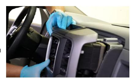
**Step 27:** Remove the four 7mm screws holding the radio in place.
