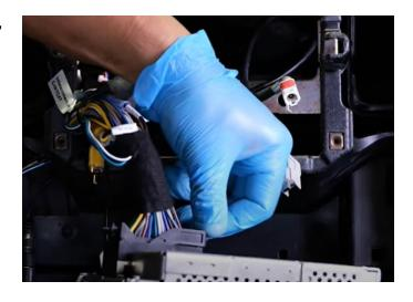
**Step 35:** Secure radio back into place with the four 7mm screws.
