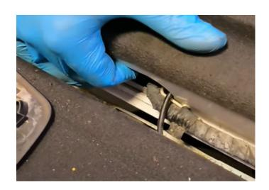
**Step 12:** Once you get to the end of the tailgate, you'll route our tailgate body harness through the factory hold going under the vehicle. Continue to route the tailgate body harness along the factory harnesses. Zip tie along the way.
