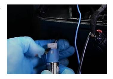
**Step 33:** Route the power connector on the EZDC behind the radio and plug it into the tailgate body harness.
