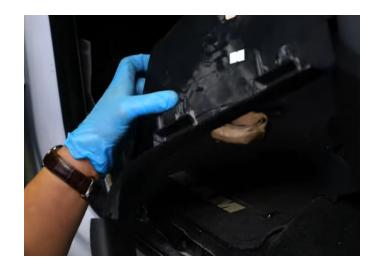
**Step 17:** Once the trim is removed you can lift the carpet and reach in to pull out the plastic grommet.
