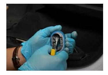
**Step 20:** Slide the plastic grommet back into place, then put the Caulking/Silicone Seal/Duct Tape into place to avoid water getting into the cab.
