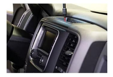
**Step 26:** Pull the bezel forward to release the retainer clips then place it to the side.
