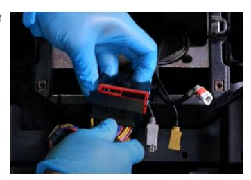
**Step 30:** Remove the plastic holding the yellow RCAs together. We will be using the female RCA going toward the radio to connect our tailgate body harness's yellow RCA too.
