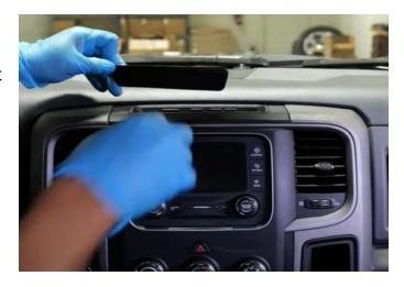
**Step 39:** Time to program the vehicle for Rear View Camera. Install the Security Gateway Module Bypass in the appropriate place. Then proceed with genie programming. This step is only needed for 2018+ vehicles. Skip this step if your vehicle is below 2018. To find your vehicle's bypass location click the link: OBD Genie Bypass
