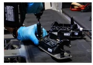
**Step 6:** Install the new tailgate handle into place. Be careful to note scratch your paint installing the handle.
