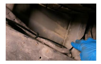
**Step 14:** Install your tailgate access panel with the eight T30 Torx screws.
