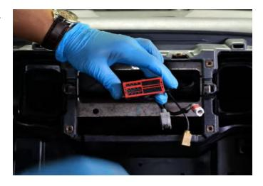
**Step 29:** Take our C4T Radio Harness and plug it into the factory 52 pin connector. Make sure to push down locking lever for secure connection.
