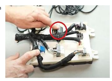
**Step 44:** Locate the LDS wire which is an Orange wire with purple stripe. Then using our posi tap or any other method you'd like, connect to the orange wire with the purple stripe. Test to make sure you got the correct wire. You'll see guide lines if correct and no guide lines in incorrectly tapped.
