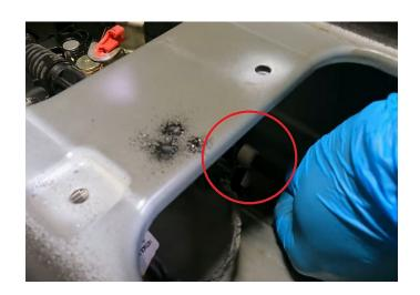
**Step 9:** Route the harness along the factory harnesses. Make your connection from the tailgate camera harness to the body harness.
