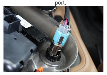
• Start the vehicle and wait 30 seconds. Insert the C-RVC programmer into the vehicle's OBDII port beneath the steering column. Once the programmer light turns green the installation is complete. Engage the vehicle into reverse to take advantage of your newly installed backup rear view camera!
