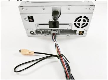
Connect the camera's power (red) and ground (black) to the EZ DC 12v Accessory Kit. You can use basic crimpers to connect the wires. The EZ DC kit can then be plugged into the backside of any <a href="mailto:switched/accessory">switched/accessory</a> 12v cigarette lighter
